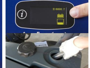
fill the tank with clean water. The clean water temperature must not exceed 40 °C
