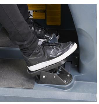
**3** Drive pedal must be released during engine cranking
