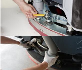
its assembly then connect the vacuum hose to the squeegee. Make proper height and inclination adjustments
