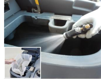
14. Wash with clean water the recovery tank and the vacuum grid. Remove and clean the debris tray.
