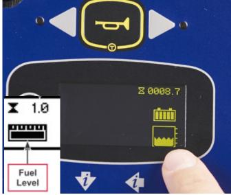
1. Check the Diesel fuel tank level / LPG bottle charge/Battery charge. In case re-fill/change the LPG Bottle / charge the batteries
