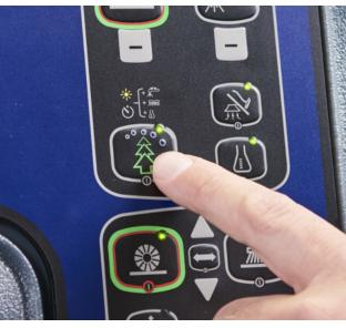
12. Press the Ecoflex<sup>™</sup> switch whenever you temporarily need a greater cleaning power
