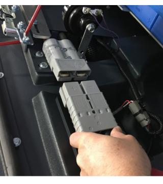
**2** For the battery version check the battery voltage and if needed recharge
