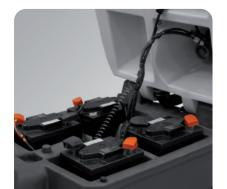
The detergent water tank serves as battery compartment, allowing the housing of great capacity batteries granting continuous working time up. Large capacity shock and acid proof polyethylene tank (110 l) improves productivity avoiding frequent refilling and idle time.
